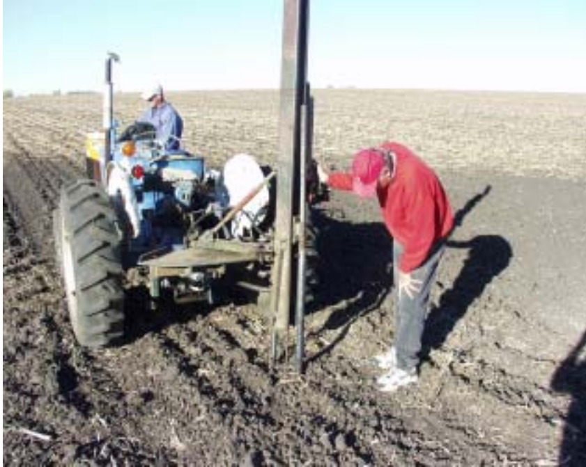
Figure 2. Collecting a soil core with a tractor probe to analyze soil horizons.
